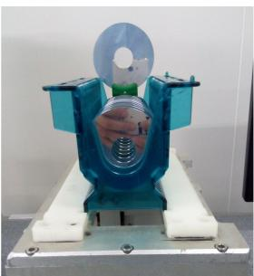
This single disc lifter tool design come in 2 difference OD size, namely 65mm and 95mm outer diameter (OD). The chassis hot shoe is suitable for common HDD shipping cassette. Operator could place the shipping cassette inside the hot shoe before lifted the disc in the cassette.
